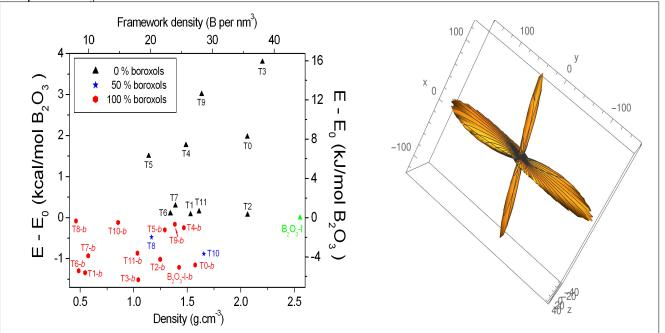
**Figure 1**. Left-Energy versus density plot showing predictions of a low energy polymorphism in  $B_2O_3$  [1]. Right – Spatial dependence of the Young's modulus of one of the new polymorph show extreme anisotropy, with two orders of magnitude between the softest direction and the hardest.
